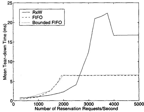
Fig. 11. Tear-down response time as a function of traffic load.
