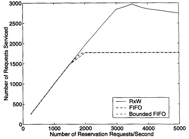
Fig. 8. Throughput of a Clearing House node as the traffic load is varied
