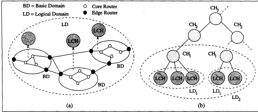
Fig. 1. (a) Local Clearing House (LCHs) associated with their basic domains that lie within a single logical domain (b) An hierarchical CH-tree with multiple levels of logical domains.
