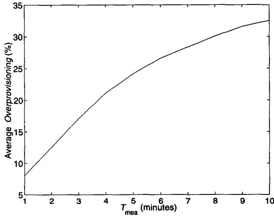
Fig. 7. Average *overprovisioning* (in %) when reservations are made based on Gaussian predictors for aggregated voice traces.
