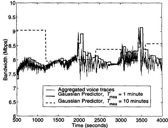
Fig. 5. Gaussian predictors for actual voice traces with measurement of 1 minute and 10 minutes.
