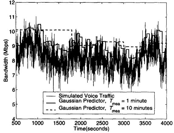
Fig. 4. Gaussian predictors for simulated voice traffic with measurement of 1 minute and 10 minutes, for  $\rho = 180$ .
